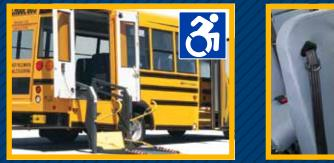
Special needs Micro Bird with double-leaf wheelchair doors offer protection on both sides of the lift, thus adding to passenger safety, while offering superior weather seal and door strength.
